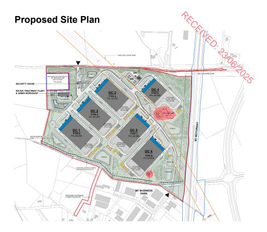
The vehicular and pedestrian site entrance is located in the north corner of the site. The entrance location has been chosen to ensure adequate sight lines can be achieved for all traffic leaving the complex. A new entrance will need to be made in the existing hedgerows to allow for this. Given the scale of the site, prominent stone wall and signage is proposed along the R409 to mark the entrance. For further details, see doc. 22217-RKD-ZZ-ZZ-DR-A-1401.
