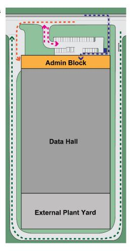
To the front of each Data Centre 2 roads are proposed for the separation of private cars and HGVs for safety reasons. A carpark is provided to the front of each data centre for those arriving via car. A rear access road is included for access to HVO compound. Rear access roads have been designed as single direction – traffic will be managed via signage. Refer to Traffic Impact Assessment for further details.
