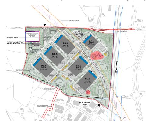
All buildings on site are stepped from north to south to follow the existing site levels. This allows for minimum cut and fill within the site. The cut from the attenuation ponds and foundations will be reused for the berms with allow for shielding of the DC buildings from the R409 and M7.
