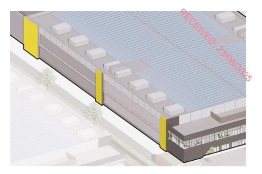
The External Plant Yard is a fully louvered wall, the provide visual screening but will allow ventilation to all electrical turbines and machinery within.
